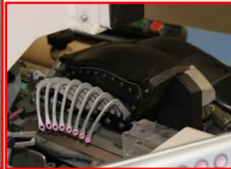
Elektronik atkı seçici step motor, normal ve atkı makası Electronic weft selector with direct weft cut device
