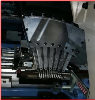
Elektronik atkı seçici step motor, normal ve atkı makası Electronic weft selector with direct weft cut device
